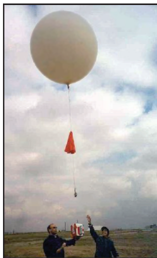
Figure 18. High-altitude balloons carry sensitive measuring devices into the upper atmosphere to check on ozone levels.
